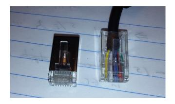
I cut the plug off the end, and then used my network crimping tool to attach the new plug. I plugged it into the radio, and the problem was solved!!! Since I already the CAT6 plug laying around, this repair was free.
